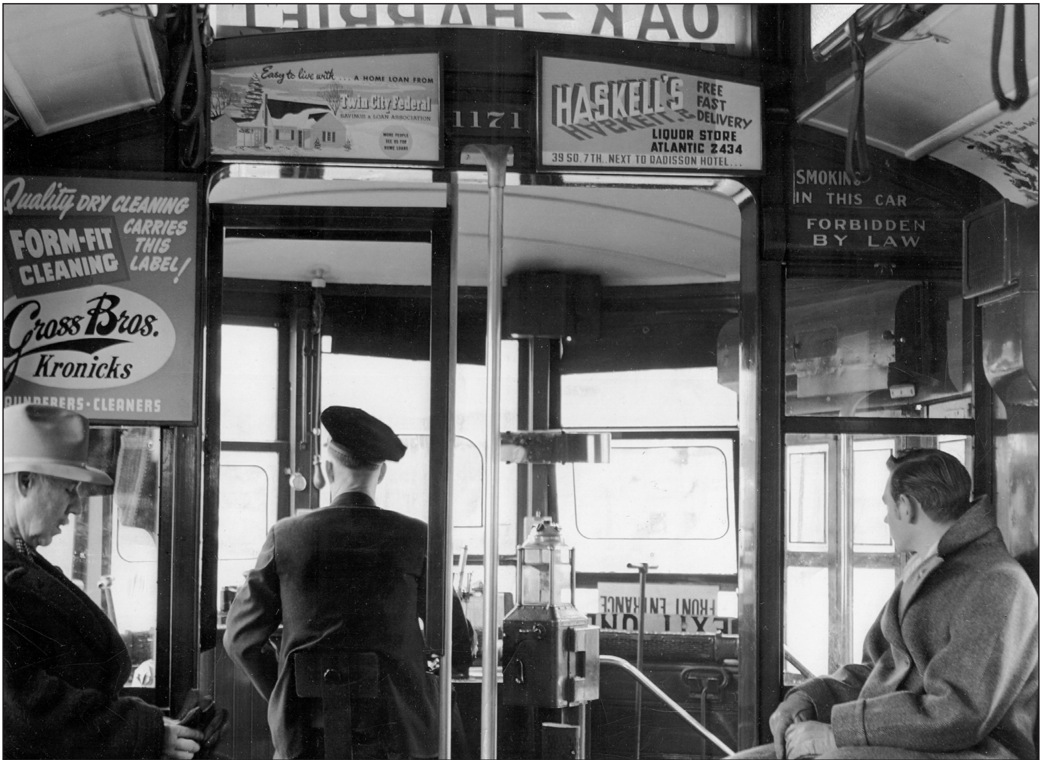
A workaday winter scene on the Oak-Harriet line. There's isinglass on the windows. Note the changer with extended token barrel mounted on the dash. The farebox has one of the caps with little coin slots that must have resulted in many coins on the floor. The ads on the bulkhead are all for local companies that still exist, though not necessarily by the same name.
